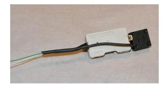
Finally, twist the white and green wires together, leaving the last inch or two untwisted. Then strip about 3/8" off the end of each wire.
