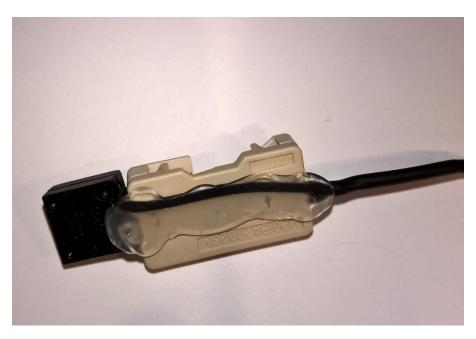
Paint the LEDs, if you haven't already. It's not entirely necessary to sand down the top of the lens, but I prefer how that ends up looking. The top can be taken down pretty quickly with 220 sandpaper, and then I like to run it on 800, to get rid of the deeper scratches.
