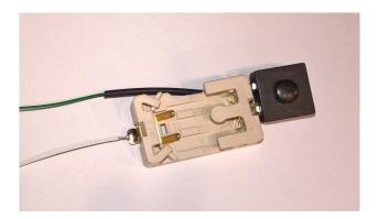
Place the shorter piece of 1/16" shrink tube over the white wire, and try to fit it over the terminal as well. If you're careful, it should just fit. Then shrink it in place.
